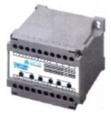
The T25-BE are electronic transducers converting reactive power and energy in three phase balanced or unbalanced systems to simultaneously produce an analogue DC output for instantaneous power signal and a digital pulse output for cumulative energy signal. Available for Unidirectional and Bi-directional.
